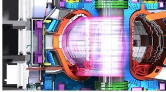
The cryogenic plant will be used to cool the electromagnets that generate the intense magnetic fields which will contain the hot plasma inside the reactor. © ITER Organization
