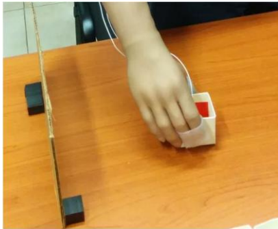
The glove can enable amputees to pick up fragile objects. Image Credit: The BioRobotics Institute, Scuola Superiore Sant'Anna, Pisa, Italy.
