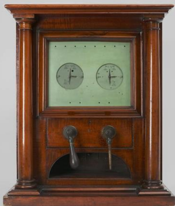
Cooke and Wheatstone Dual-Needle Telegraph
